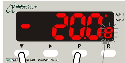
Press and hold (▼) and (P) simultaneously for 3 seconds
