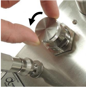
Pressure Regulator fully closed anti-clockwise
