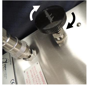
Needle Valve fully closed clockwise
