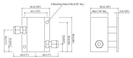
Note: The Assembly is shown with 1/4@ OD tube fittings. The dimensions across the tube fittings will vary for all other size fittings.
