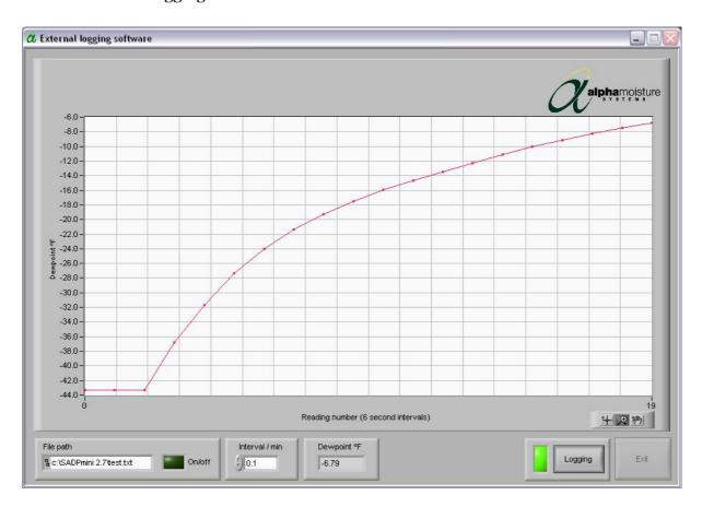
The External Logging screen will automatically communicate with the attached SADPmini and update the graphical and digital displays. The graph has auto-scaling axis. The Y-axis shows the moisture level in the current engineering units of the SADPmini. The X-axis shows the number of readings and the interval between each reading. Approximately 8000 readings can be displayed on the graph before the display automatically scrolls
