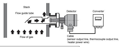
Replacement of the existing detector ZFK2 with the detector ZFK8:
