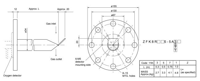
(4) Flow guide tube (For corrosive gas)
