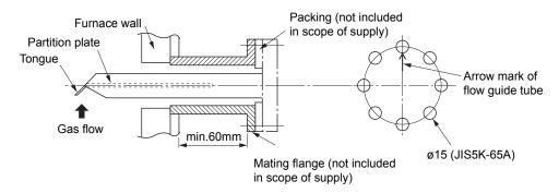
2 When exhaust gas temperature is 200°C or higher and gas flowing velocity is fast As illustrated below, till the partition plate inside the flow guide tube 45° to the gas flow and mount the tube so that the tongue turns to a down-steam direction relative to gas flow.
