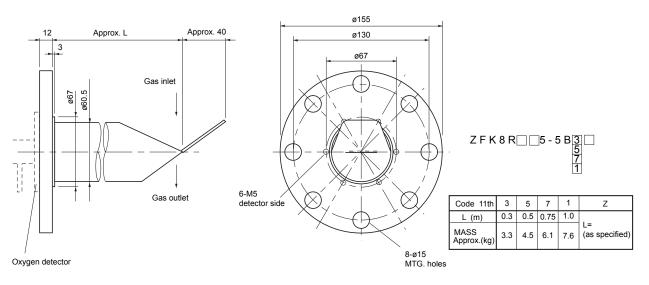
(5) Flow guide tube (with blow down nozzle)
