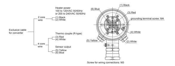
Connect the protective grounding to one of the two terminals in the figure below. (Class D (Class 3) grounding, grounding resistance:  $100\Omega$  or less)
