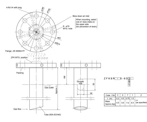
(7) Flow guide tube (for high particulate with cover)
