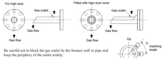
Set the inserting angle within a range of 0 to  $+45^{\circ}$ .
