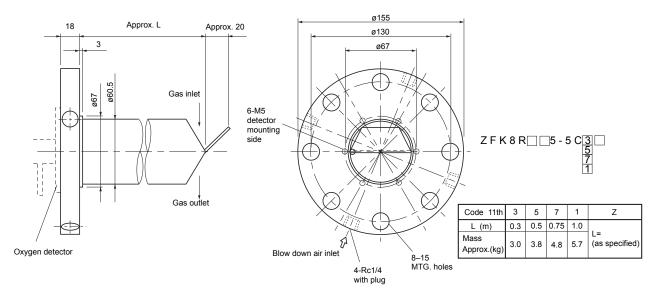
(6) Flow guide tube (for high particulate)
