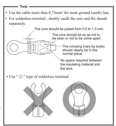
Attach the solderless terminals to the grounding terminals with them between the tooth lock washer and screw with washer.
