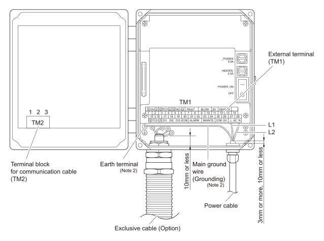
Note 1: Fix the exclusive cable ( $O_2$  sensor input /  $O_2$  sensor thermocouple input) with the cable gland so that its sheath is 10 mm or less.
